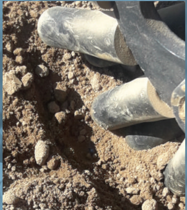
Fig. 11. Finger press wheel disrupting seed placement in dry conditions.
