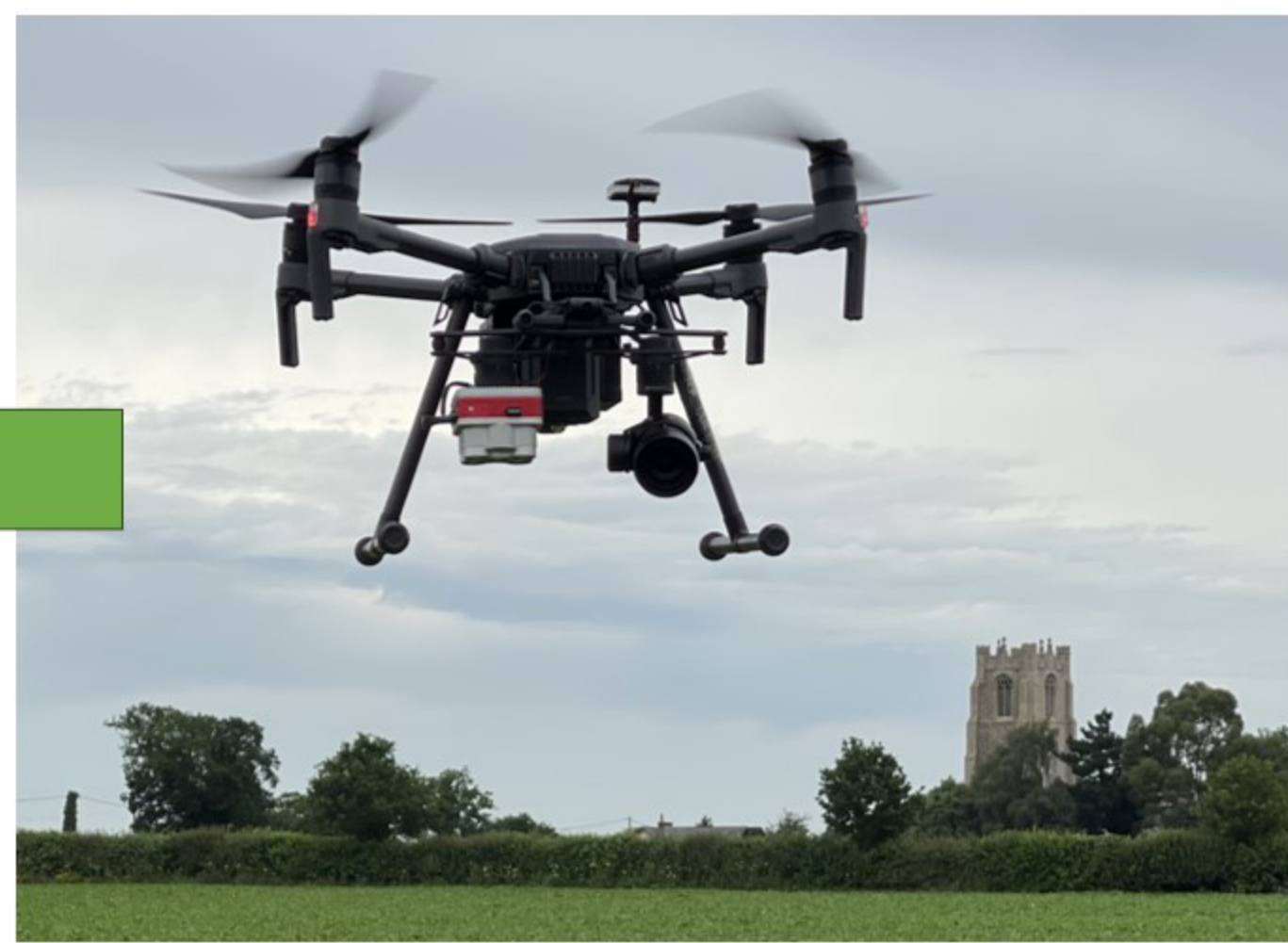
Once VY symptoms appear then the trial is regularly flown over by UAV. On-board it carries a range of cameras which capture full colour (RGB), thermal and multispectral imagery.
