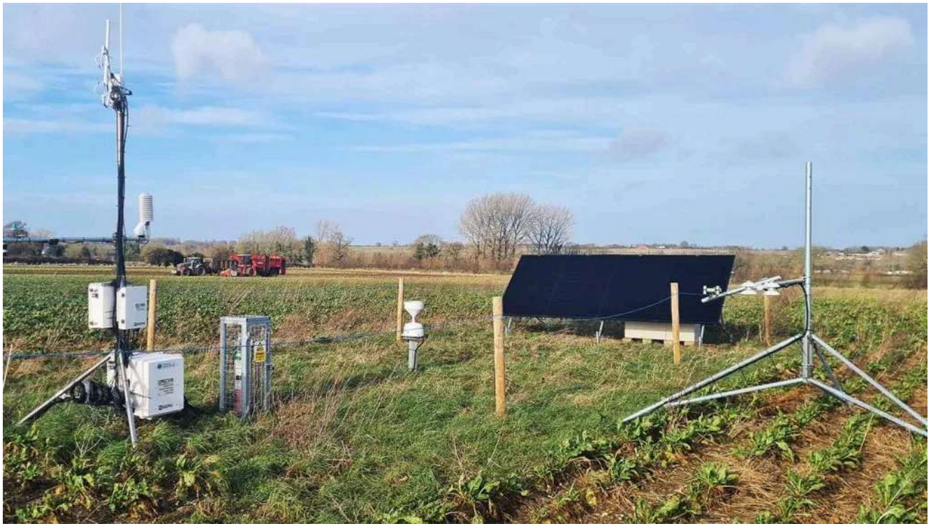
Flux towers at Morley Farms comparing the carbon absorption or emissions of beet under different management systems.
